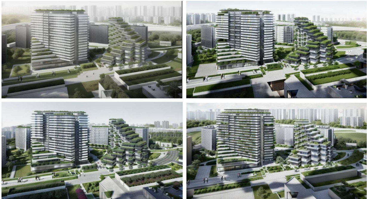
Fig. 12: Labbe, J.: Diverse AI-tools deployment at a multi-level design development. Luka Development Scenario, Prague . MS architekti, Prague. 2024. author's archive. The volumes of the buildings = the geometry of the model stabilized by ControlNet, Stable Diffusion delivers options for the architectural forms of the buildings. The complete workflow in figures 3 to 11 and in the text, section (2) of the paper.
